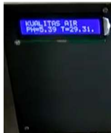
Figure 4. Display of water quality data (water temperature and pH) on the LCD E-Ox Level
